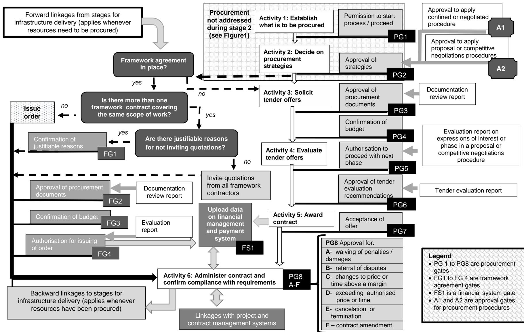
Figure 6: Control framework for a procurement system based on ISO 10845
